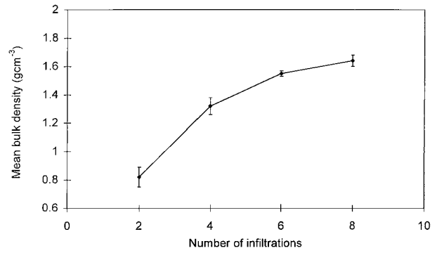
Figure 3 The change in the mean bulk density of the C/SiC-based composite with the number of infiltration cycles.
