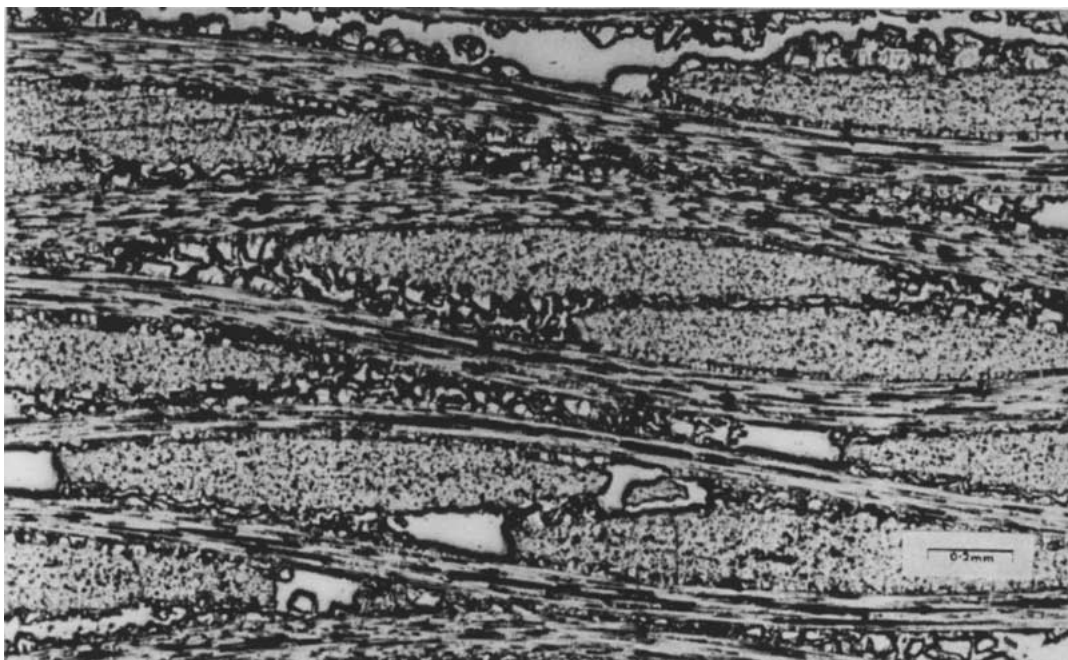
Figure 8 Optical micrograph of a cross-section of the C/SiC-based composite after 6 infiltration cycles.
